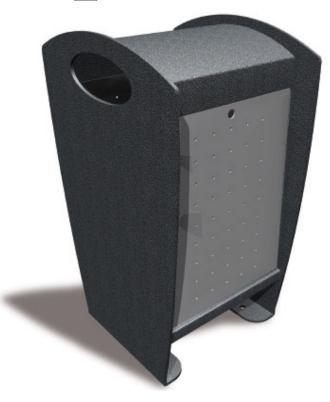
Painted steel mounting system and lid opening, thickness 8mm - painted perforated aluminium liner, thickness 3mm with 6mm rounds. Capacity 54 litres. Liner emptied by removal at the side - Lockable liner RAL 7004 - Fixing on to a concrete block
