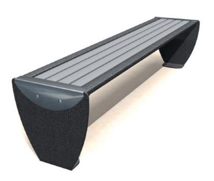
Seat comprises 2 painted steel slats 50x25x2,5 mm, and 4 pultruted polyester slats (polyester composite/fibre glass) 58x25x3 mm, RAL 7004. Black polyester powdercoated steel base, thickness 8mm - Stainless steel brackets and fixings - Fixing on to a concrete block
