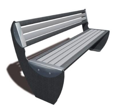
Seat comprises 2 painted steel slats 50x25x2,5 mm, and 4 pultruted polyester slats (polyester composite/fibre glass) 58x25x3 mm, RAL 7004. Seat back comprises 2 painted steel slats 50x25x2,5 mm, and 2 pultruted polyester slats (polyester composite/fibre glass) 58x25x3 mm, RAL 7004. Black polyester powdercoated steel uprights, thickness 8mm - Stainless steel brackets and fixings - Fixing on to a concrete block
