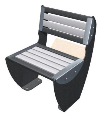
Seat comprises 2 painted steel slats 50x25x2,5 mm, and 4 pultruted polyester slats (polyester composite/fibre glass) 58x25x3 mm, RAL 7004. Seat back comprises 2 painted steel slats 50x25x2,5 mm, and 2 pultruted polyester slats (polyester composite/fibre glass) 58x25x3 mm, RAL 7004. Black polyester powdercoated steel uprights, thickness 8mm - Stainless steel brackets and fixings - Fixing on to a concrete block
