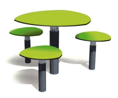
Table and seat tops manufactured from 13mm thick compact - Black polyester powdercoated steel posts for table and stools. Table: diameter 125mm, thickness 2.5mm Stool: diameter 102mm, thickness 2mm. Stainless steel fixings protected by ployamide anti-vandal caps
